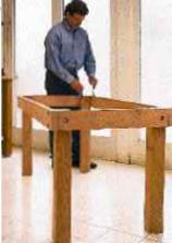
and bolts with socket wrenches and let glue dry overnight. 11. Lower top onto base to check fit, then remove and sand and seal each
