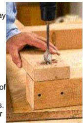
using a 3/8-inch bit, drill holes through the end piece and each leg. Switch to1-inch paddle bit (shown in photo) and use these holes as guides to drill a 7/8-inch-deep hole in each leg back and in the outside face of the end piece. Repeat for opposite end.
