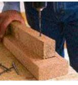
and cut two 2-by-2 ledgers to measure 1/4 inch less. Center and align each 2-by-2 on line marking tabletop's thickness on each 2-by-4 side piece; secure with five 21/2-inch deck screws.
