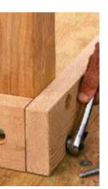
of the end boards before drilling a pair of holes centered over leg and 3/4 inch from edges of each side board. Loosely assemble base upside down with glue, hex bolts, nuts, and washers. 8. Overlay one end piece flush with tops and sides of a pair of legs. Center and.
