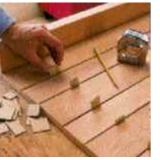
by-4s and 11 1-by-3s flat between them. Insert cardboard spacers between boards to determine the tabletop's length. 2. Butt each remaini ng 2by-4 against one end of the
