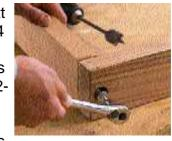
Center and drill pilot holes through sides into ends with 1/8-inch drill bit. Switch to 1inch paddle bit and drill 7/8inch-deep holes into sides. Assemble frame using glue and lag screws with washers.
